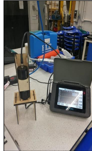
Figure 5: Ultrasonic Velocity Equipment Set-Up Using Proceq Pundit PL-200
