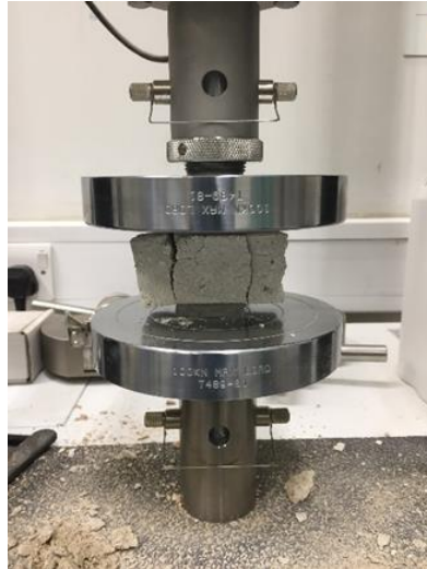
Figure 8 OPC and lime putty sample 1 showing fracture after completion of compressive testing
