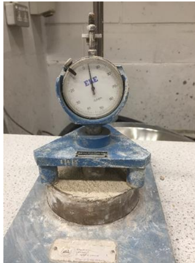
Figure 4 Drop Ball Test of Lime Putty Mix
