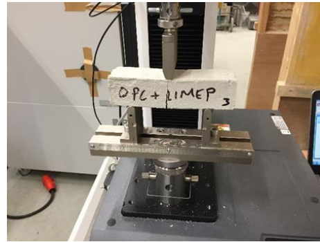
Figure 6 OPC and Lime Putty Sample 3 Flexural Testing in accordance to BS1015-11:1999
