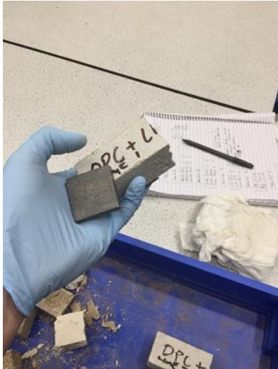
Figure 7 Compressive testing on OPC and lime putty sample 1
